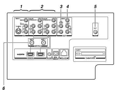
VIDEO 1 IN — Composite video and analog audio inputs plus optional S-video inputs for connecting devices with composite video or S-video output.
